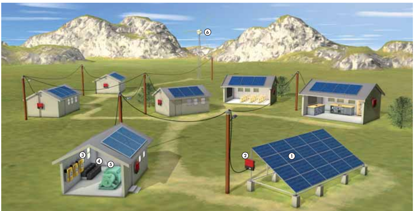
Components: 1. Solar generator, 2. SUNNY BOY, 3. SUNNY ISLAND, 4. Batteries, 5. Diesel generator, 6. Wind power plant
